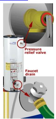
Open all the hot-water spigots in the house, and turn on the cold-water inlet to the tank.
